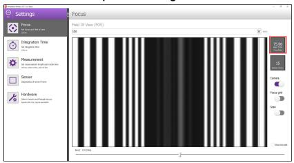
You can make use of the "**Focus rate**" value to get the best focus. Adjust manually the lens and until you reach the highest focus rate and the lines are sharp.
